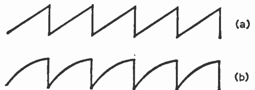
Fig. 2 (below): The ideal and actual waveforms produced.
