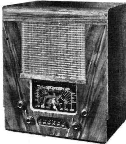
One of the new McMichael all-wave superhets with push-button tuning.
