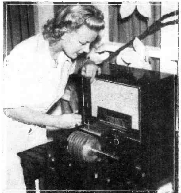
Manufacturers go to great pains to make certain that mechanical parts will not break down. Here is a Philips' Tester which operates the push-buttons, pressing each button 160 times at the rate of 23 times a minute.
