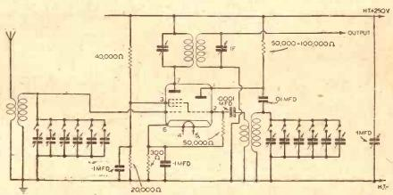
Fig. 3.—A superhet unit with push-button tuning in both circuits.
