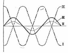
Fig. 2.—Voltage, current and flux curves in a mains transformer. I=Applied primary volts: II=Magnetising current: III=Flux: IV=Back E.M.F. of self-induction.
