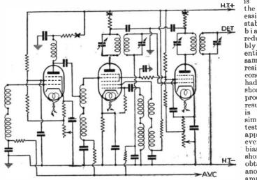
This skeleton diagram of a hypothetical H.F., F.C., I.F. circuit shows the condensers and resistors referred to in the text. Crosses indicate suitable points at which a milliammeter may be inserted to test for self-oscillation.
