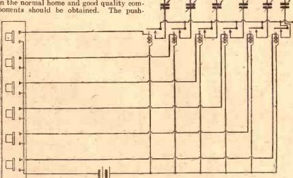
Fig. 5.—A remote control push-button unit, with relays for each station.
