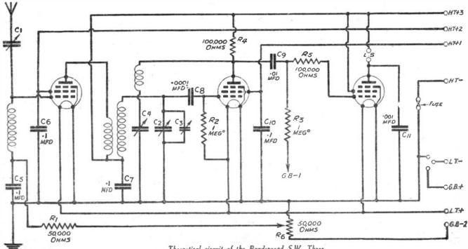
Theoretical circuit of the Bandspread S.W. Three.
