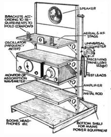
Fig. 4.—Another form of experimental rack, useful where space is limited.
