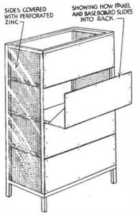
Fig. 2.- A box rack structure. With this method complete protection is given to all apparalus.
