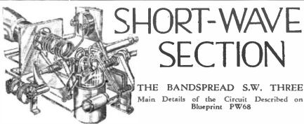
1936 we described a very efficient three-valver for short-wave use, in which the bandspread system of tuning was employed. The circuit is given below, from which it will be seen that an H.F. stage is employed, with the bandspread tuning in the detector stage. R.C. coupling is employed between the detector and output valve, and rentydes. detector and output valve, and pentodes are employed in all three stages.
