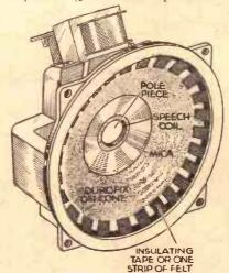
Method of improving the tone of a moving-coil speaker.
