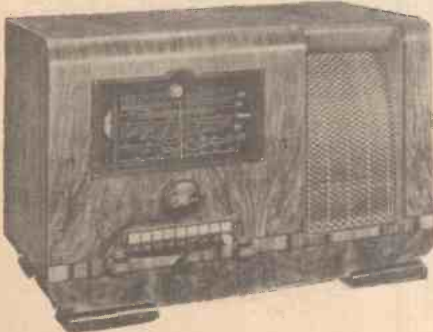
Push-button tuning is included in this new H.M.V. receiver. It is shown on Stand No. 47.
