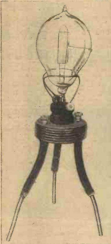
Sir Ambrose Fleming's thermionic valve. This also shows the earliest valvholder improvised in the Swan laboratories.
