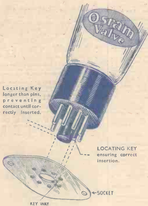
Diagram showing self-locating feature of "International" Octal Base.
