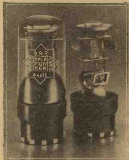
"Magic Eye," or visual tuning indicator with side contact base.
