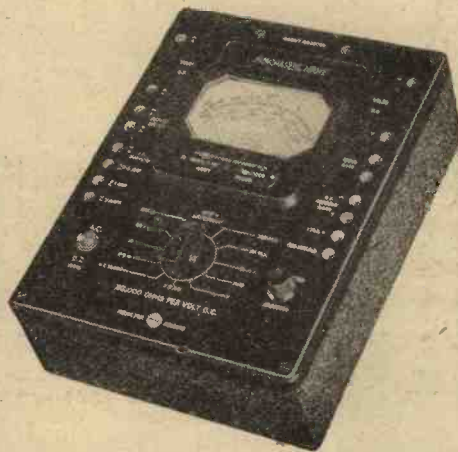
A comprehensive Analyser from the range of Weston measuring instruments to be seen on Stand No. 167. This has been designed so that it may be used for television servicing in addition to ordinary radio purposes.
