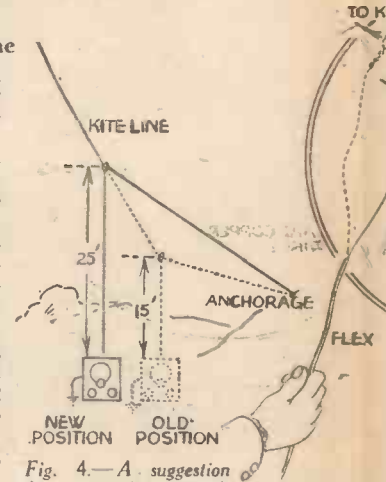
Fig. 4.—A suggestion for using short aeriels for S.W. work.
