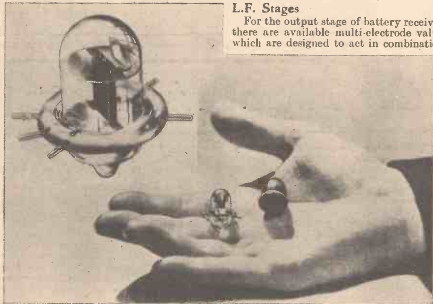
One of the Acorn Midg-st valves shown in comparison with an acorn.
