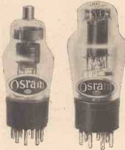
Two of the new valves; on the left the H42 and on the right the N42
