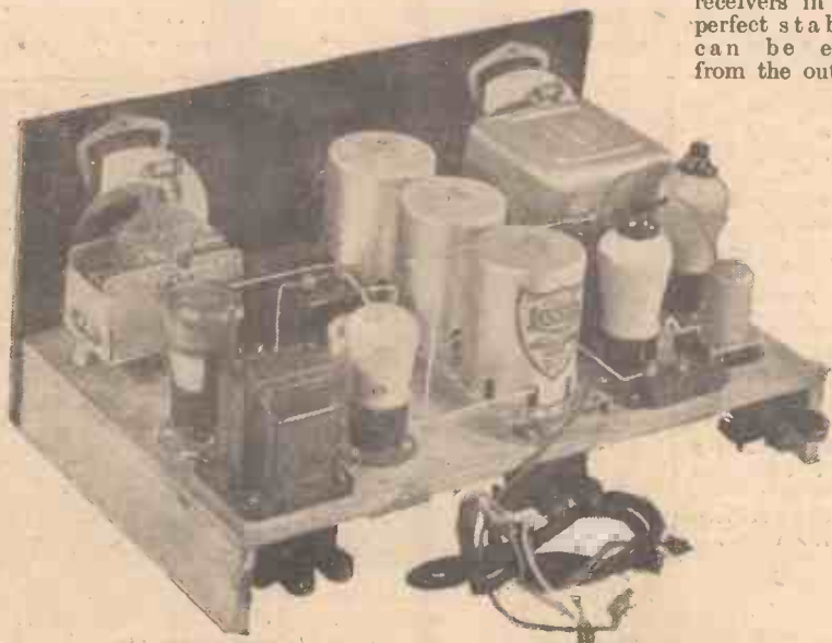
An early design, using four valves, which may be compared with the illustration above. This is the famous Fury Four receiver.
