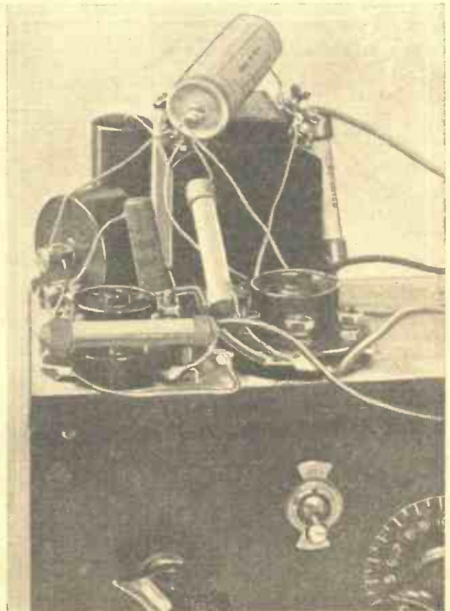
Fig. 3.—This illustration shows the detector and output stages, and the compact arrangement of the remaining components.
