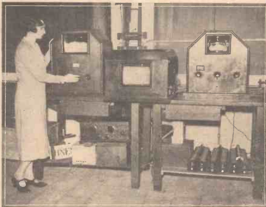
A television receiving set of the Fernseh A.G., which belongs to the well-known Goertz Company, and which is used by the German Reichspost authorities for experiments preliminary to the introduction of a public television service.
