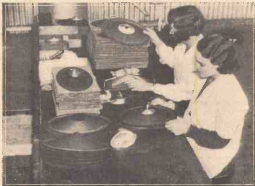
Fixing the special metal centre on the cones for "His Master's Voice" high fidelity loud-speakers.
