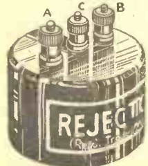
TRANSMISSION LINE FROM AERIAL REJECTOSTAT CONNECTS ACROSS A & B. EARTH VIA SHIELDING TO C
