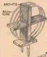
A short-wave coil and a novel form of adjustable coil-holder.
