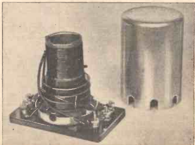
Fig. 2.—A home-made coil in which the reaction winding may be moved or rearranged in order to obtain better reaction effects.
