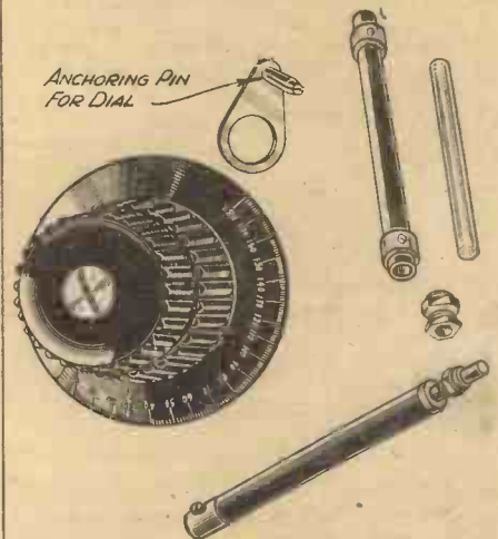
Fig. 3.—A removable slow-motion drive and some examples of extension spindles.
