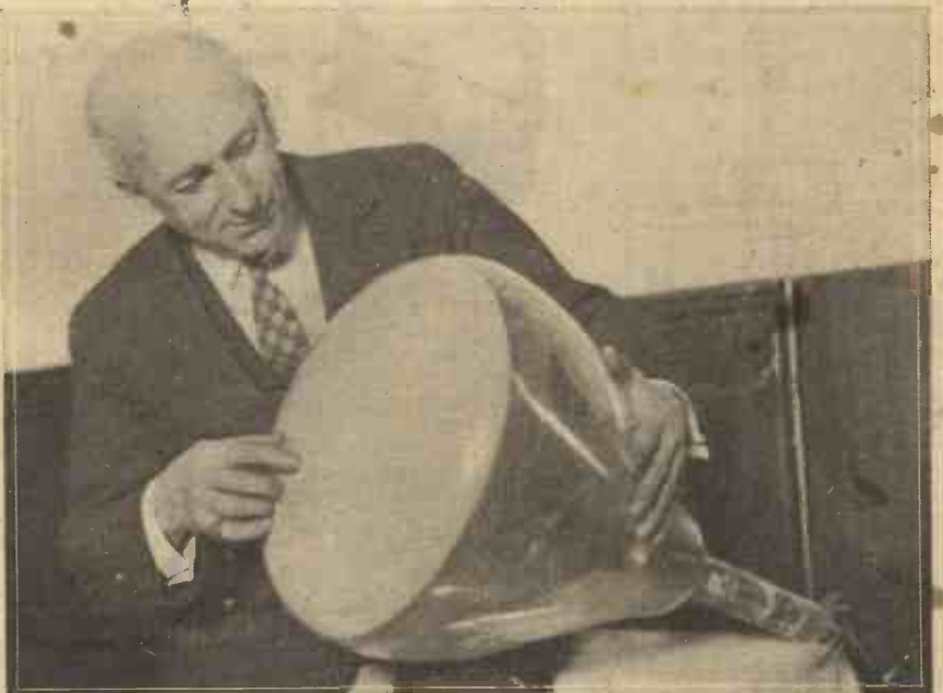
Here is the largest cathode-ray tube made in England, with Dr. J. B. Kramer, of the G.E.C., who have just produced it, indicating the frosted end upon which a 12in. x 9in. picture of any colour is viewed. No other apparatus save amplifier comprises the picture receiver, while at the studio a special camera—which develops the artist's photograph immediately it has secured it, projects it to the transmitter, and then re-sensitises its endless film.
