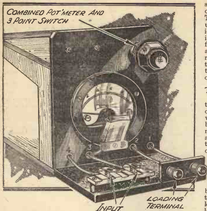
Fig. 4.—This sketch shows the front of the instrument and the connections to the input and loading terminals.
