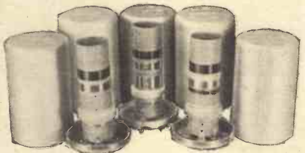
Air-core coils can also be efficient, and here is a group of Bulgin coils, with screens.
