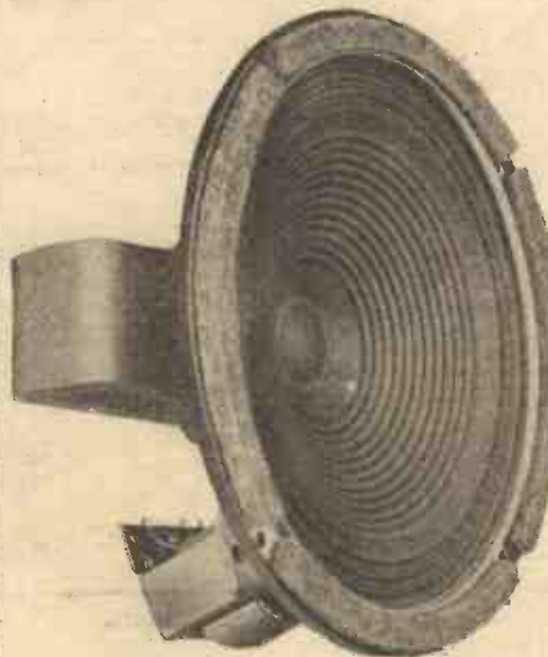
One of the permanent-magnet moving-coil speaker units from the British Rola range.
