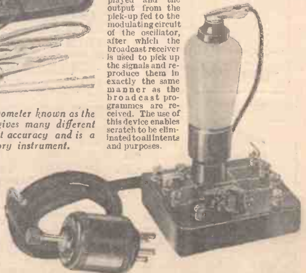
The Avodaptor which enables readings to be taken whilst the valve is working in a set. The plug on the left is inserted in a valveholder in the set in place of the valve and the valve plugged into the adaptor. It is used in conjunction with the Avominor above.
