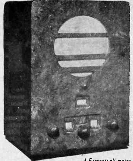
A Ferranti all mains superhet of pleasing design and efficient workmanship.
