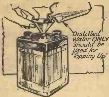
Fig. 4.—Never add acid when "topping" up accumulators.
