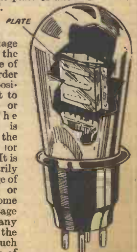
Fig. 5.—Valve cut away to show the plate.
