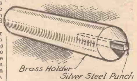
Fig. 4.—Punch for making the holes.
