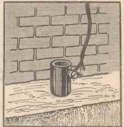
Fig. 4.—Look to the earth connection.
