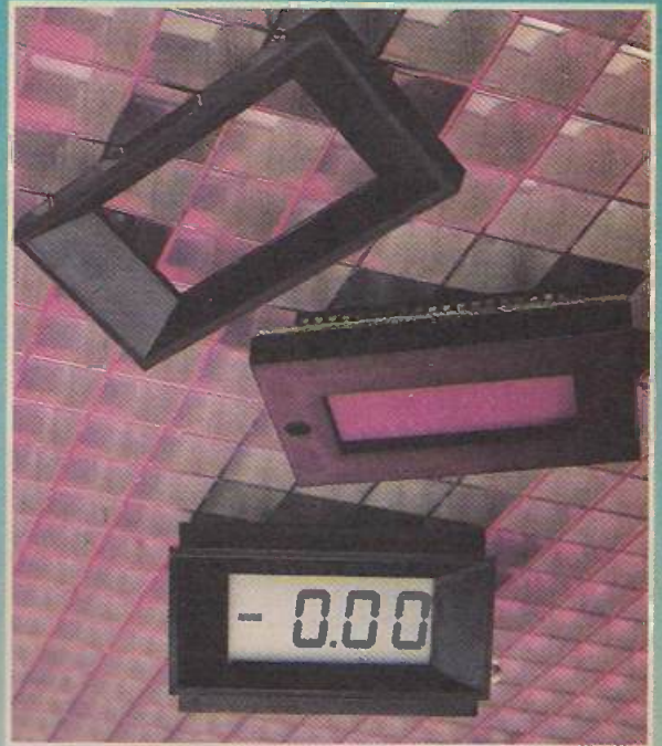
Incorporating the ICL7106 a-to-d converter, this digital panel meter has a full-scale input sensitivity of 200mV and a high input impedance of >100MΩ.
