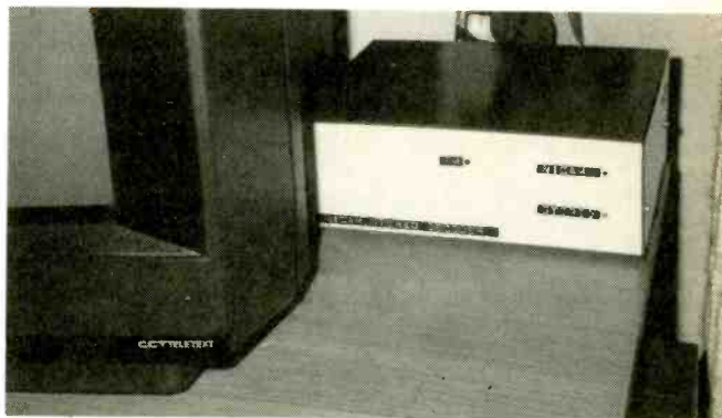
The Nicam stereo decoder unit sits inconspicuously beside the main receiver.
