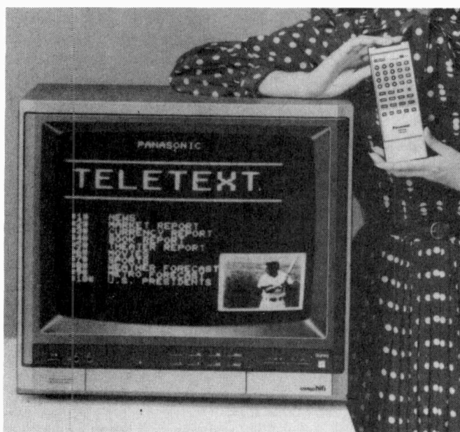
Amongst the features of Matsushita's multifunctional digital receiver is colour picture within a picture, shown here.
