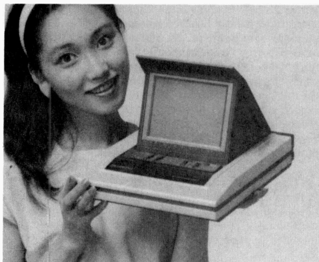
Matsushita's rear-projection colour portable receiver.
