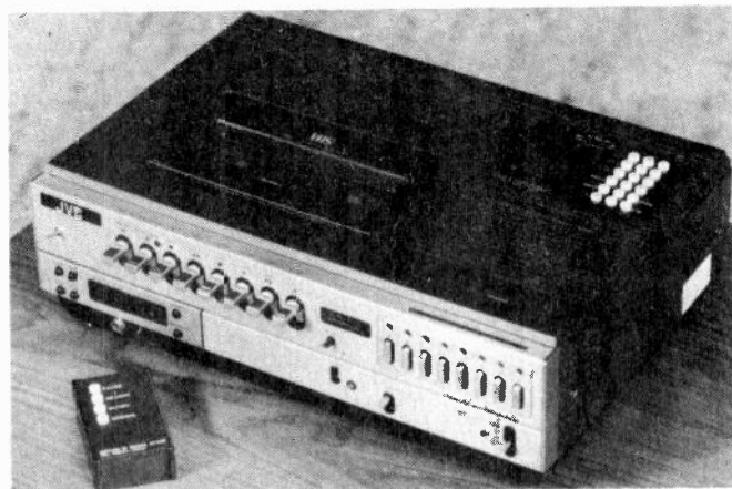
A JVC VCR incorporating the Selman up-dating modification with remote control.
