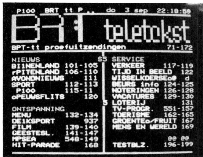
The BRT (Belgium) teletext index page 100, photographed by Jeff May (Colchester) on the screen of his unmodified Philips colour receiver (KT3 chassis). The transmission was on ch. 43, using an aerial directed at Dover.
