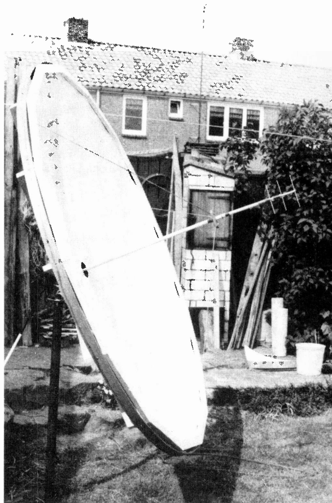
The 2-metre dish used for ATS satellite reception by Peter Jansen, Holland.
