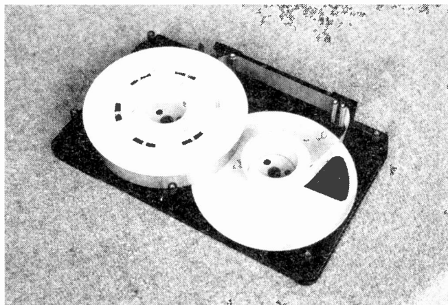
The videocassette, shown with the lid removed.
