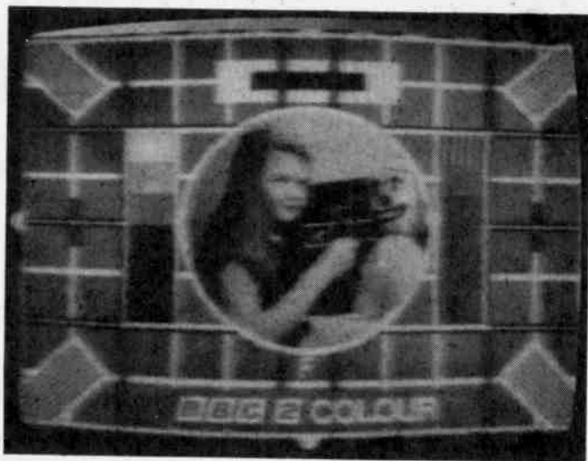
Test card F taken with 2 seconds exposure time at f22 with a \times 4 neutral density filter. All photos taken with 125 ASA film.
