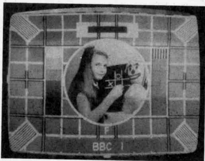
Exposure time for this photograph was \frac{1}{30} of a second at f5.6 . Note brightness variation due to an incomplete frame being recorded.
