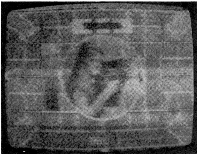
For low signal conditions, this is the result of photographing exactly what the camera sees. This was taken at \frac{1}{30} of a second at f5.6.
