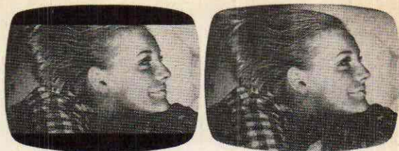
Fig. 1: Aspect ratios for cinema and television. The effect of using a hard-mask in the camera when the film is shown on television is illustrated on the left.
