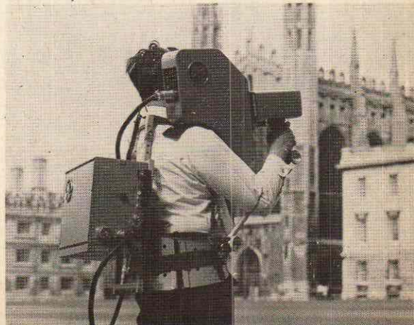
The Pye/Philips/CBS Minicam colour television camera in operation at Cambridge.
