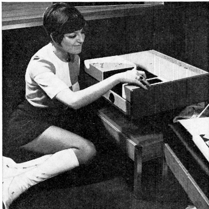
The EVR Teleplayer—it measures only 18 in. square by 5 in. high, and weighs just 35 lb, but can hold a one-hour film cassette and play it through a normal 625-line TV set. It should be available by mid-1970, costing just under £200.
