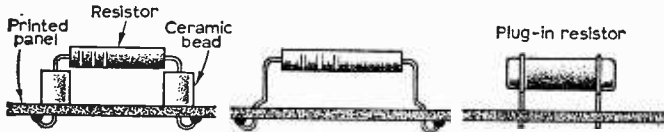
Fig. 12—Spacing resistors off the panel.
