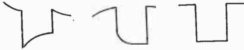
Fig. 11 (left).—Waveform shows poor L.F. response. Fig. 12 (centre).—Waveform shows poor H.F. response. Fig. 13 (right).—Perfect waveform.
