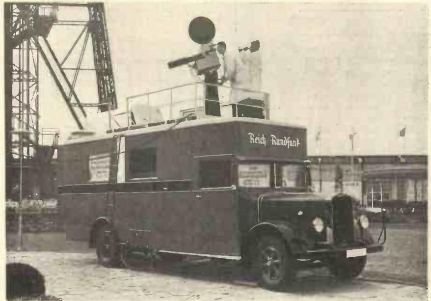
Fig. 5.—The mobile van containing the Fernseh A.G. intermediate film camera and associated apparatus.
