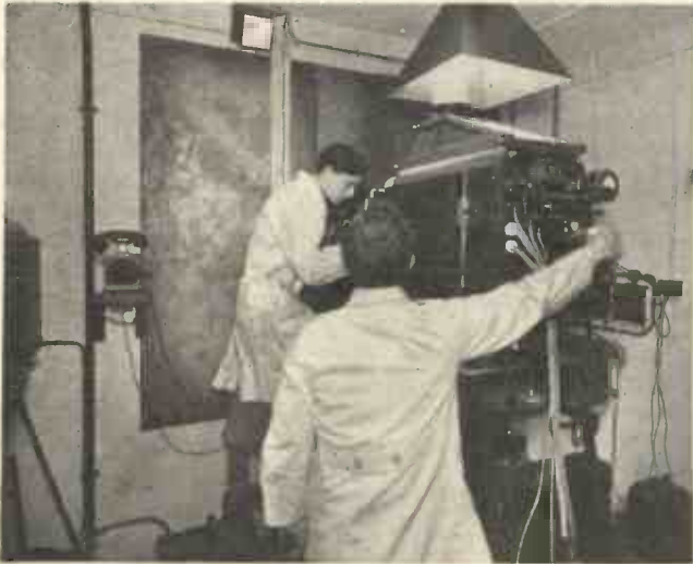
Fig. 1.—The arc lamp and rotating-disc mechanism of the Baird high-definition light-spot scanner
