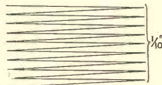
Fig. 2.—Showing how the picture is scanned.
