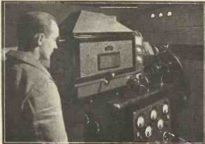
The Fernseh A.G. Light Spot Scanning Transmitter for 180 lines, 25 images per second, and 40,000 points, as delivered to the German Post Office.
