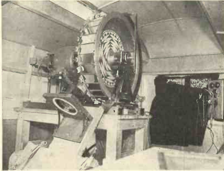
Fig. 3.—The large mirror-drum scanner and driving motor used in connection with three-zone outdoor television.
