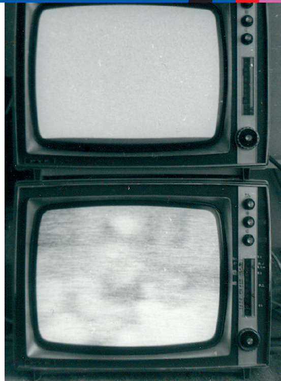
A normal and reduced vision I.F. bandwidth comparison. The top receiver is fed directly from an incoming noise-level signal while the lower set displays the effect of bandwidth reduction via an external tuner
