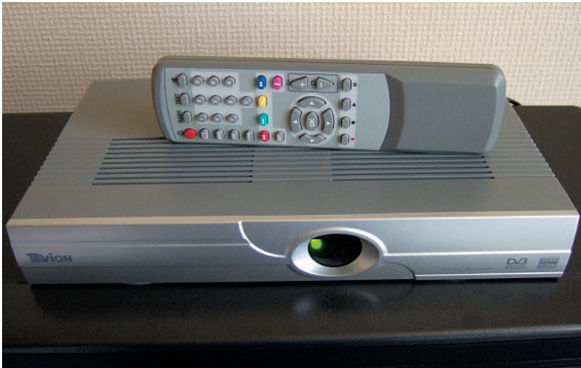
Fig. 3: The Tevion STB715 is a comparatively recent 'budget' receiver with a 7-day EPG and the ability to load channels manually
