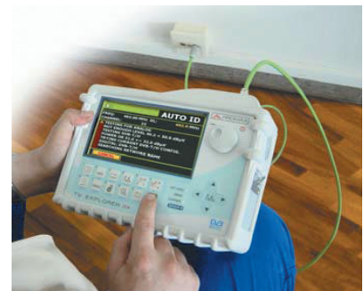
Testing & recording the quality of signal at each outlet plate
