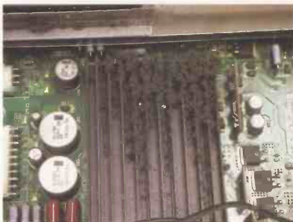
Heat sink. If fluff and dust is concentrated in one place this blocks heat dissipation and can lead to the component underneath failing
