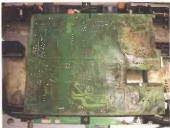
This panel was overheating. Panel was repaired by bypassing the protection circuit so it didn't turn off anymore. It eventually overheated to the point where it caught fire
