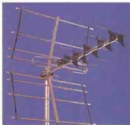
This high-gain aerial is one way of ensuring quality and consistent reception
