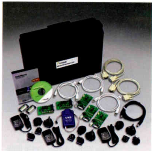
Fig. 1: Typical ZigBee development kit from Freescale Semiconductor.
