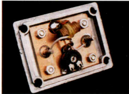
Internal view of the HS Publications Band I notch filter type CF70.
