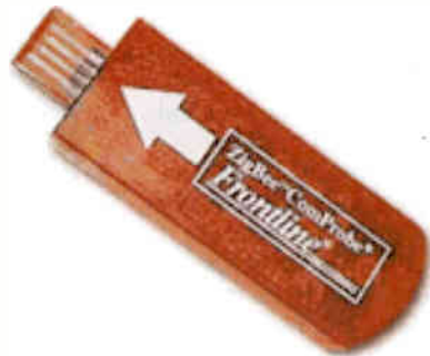
Fig. 6: The finger-sized ComProbe for ZigBee sniffing.
