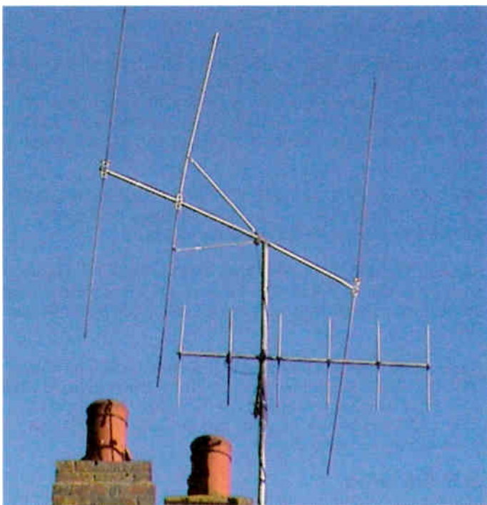
Vintage aerials. A tilted three-element Telerection Band I array and a six-element Band III array still up amongst the chimney pots. See more on wavefront tilt. Photo courtesy Hugh Cocks.
