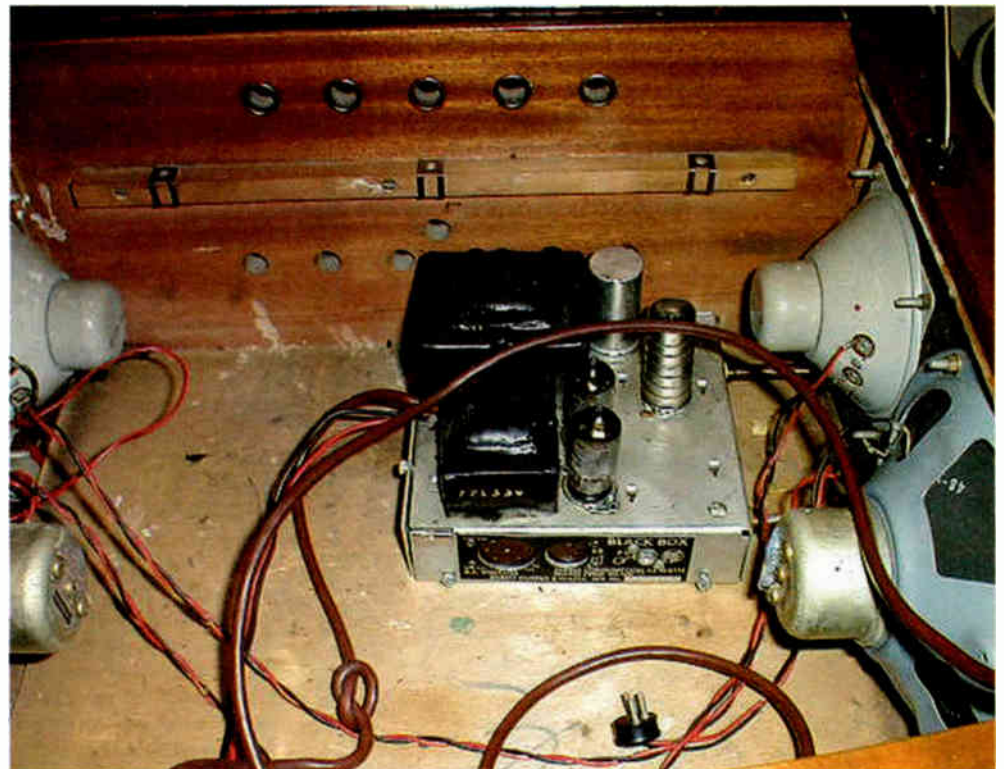
The amplifier refitted in the Black Box cabinet.
