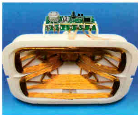
Photo 4: The double-mussel rectangular-coil deflection yoke assembly developed for the 32in. widescreen Cybertube+ SuperSlim CRT.
