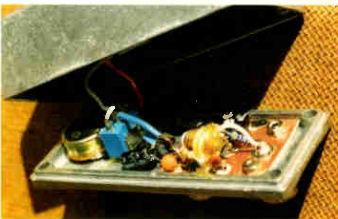
Internal view of the prototype HS Publications varicap-tuned notch filter for Band I.
