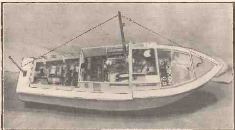
Fig. 22.—Overall view of radio-controlled cabin cruiser using the pulsed pulse system.
