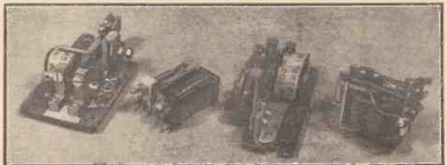
Fig. 20.—Types of relay used in this equipment. Left to right: Siemens high speed relay (1 coil \times 145 \Omega ); miniature double pole changeover relay of ex-W.D. origin (coil resistance 170 \Omega ); Siemens high-speed relay (2 coils \times 1,700 \Omega each); double pole changeover relay (ex-W.D.) rewound with 34 s.w.g. enamelled wire.
