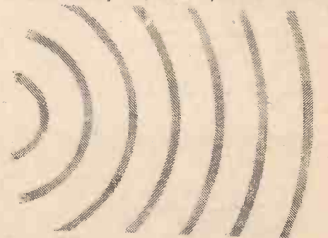
Fig. 3.—Wide beam of short frequency modulated pulses is emitted by most bats while hunting. Each pulse is about 1.5 ft. long. Beam is fixed with respect to bat's head.
