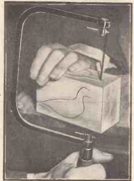
Fig. 6.—Method of sawing block with coping saw.
