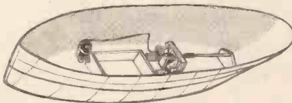
Fig. 2.—The completed hull with fitting for battery.
