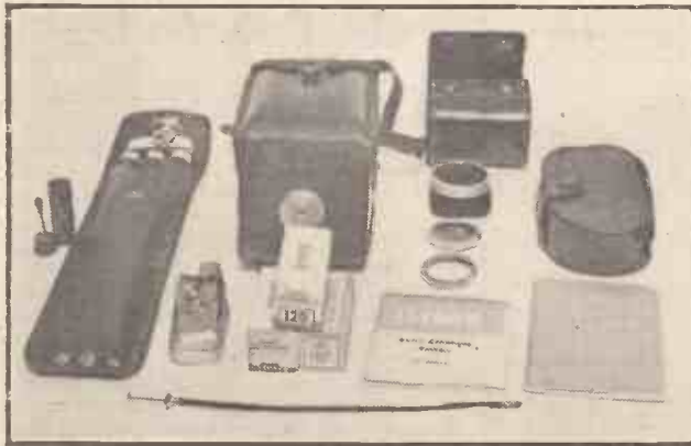
Fig. 1.—A typical kit for holiday photography, comprising camera in ever-ready case, tripod, cable release, self-timer, lens brush in case, spare films, lens-hood, filters and case, cleaning tissues, exposure meter and record book.
