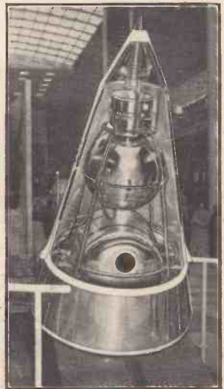
In the photograph above can be seen a model of Sputnik II. This was the type of rocket inside of which the Russian dog "Laika" was projected into space last year. The satellite weighed 1,120 lb. and was 15 ft. long. The model is being exhibited in the Russian pavilion at the Brussels Universal and International Exhibition.
