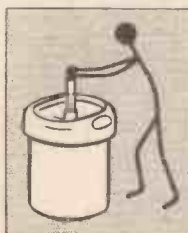
Bleach/harden for 10 mins. Wash for 5 mins.
