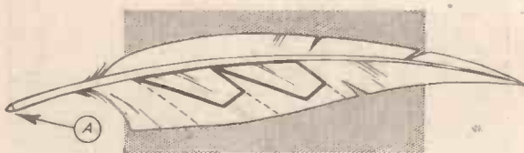
Fig. 20.—How two or three flights might be cut from one turkey feather.
