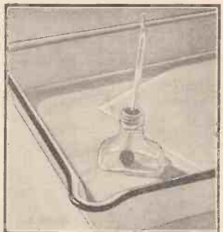
Fig. 21.—A photographic thermometer (dish development).
