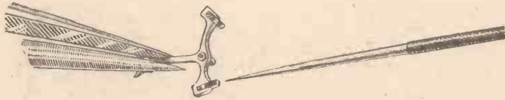
Fig. 9.—The pallet should be held in a pair of tweezers and the pallet stones examined to see if they are loose.
