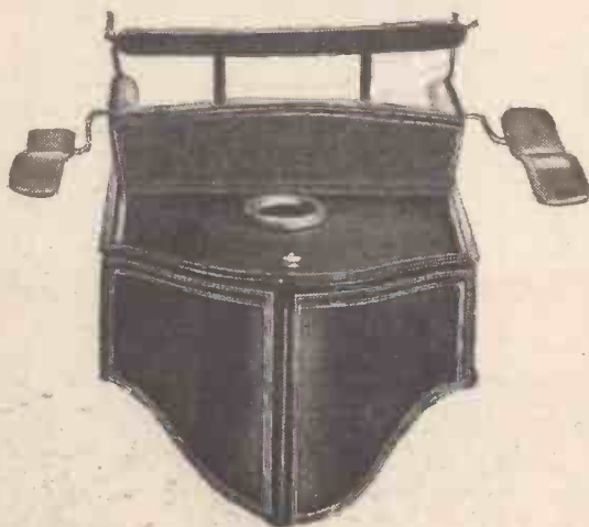
A rear view of the body. The two swing doors enclose the power unit.
