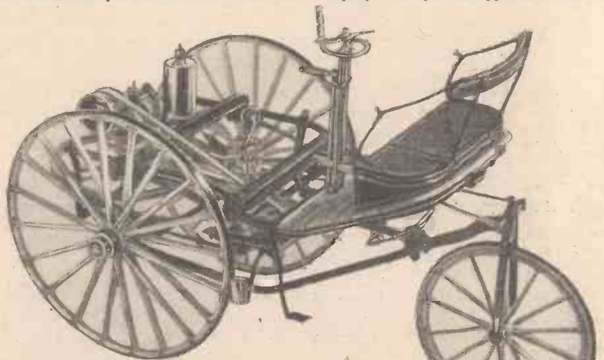
A three-quarter front view of the chassis of the model of the 1888 three-wheel Benz car, with single cylinder, four-stroke, water-cooled engine, with horizontal flywheel. At 250 r.p.m. the engine develops 2 h.p. The wheels are iron-tyred, and the drive was by belt from a pulley driven by the crankshaft, the belt driving on to a combined two-speed differential gear. The model was made by Mr. F. J. Camm.
