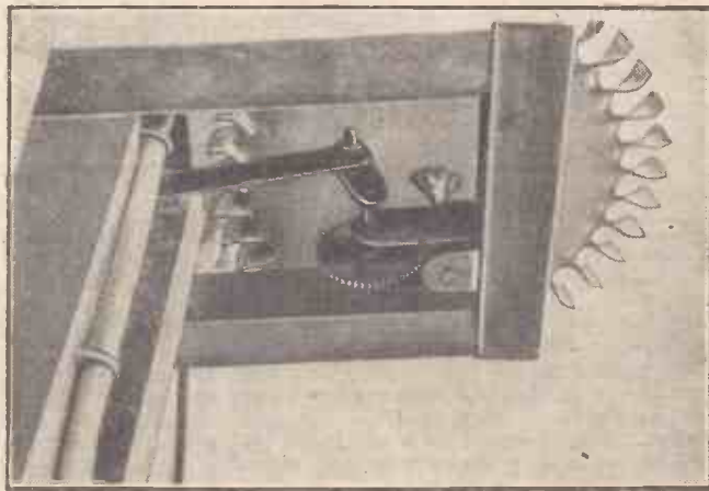
(Above) An underside view of the turbine wheel showing crank and linkage. (Below) A view with the turbine wheel lifted off the bracket to show crank and linkage.
