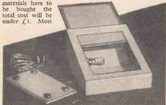
The safelight with screen withdrawn and endplate removed.
