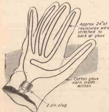
Fig. 1.—The wire stitched to the gloves.
