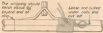
Fig. 6.—The method of whipping.
