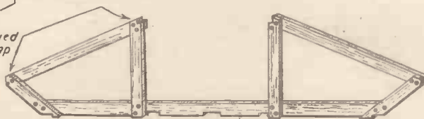
All bottom joints only temporarily screwed until final assembly
