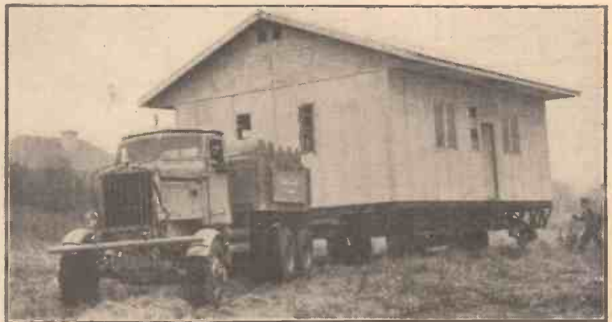
In response to a request from an oil company operating in the Middle East, Messrs. Maycrete Ltd., in conjunction with G. H. Burgess & Co., have produced a fully mobile camp building for use in connection with oil prospecting. The illustration shows the building, known as the "Supalite" Mobile House, being tested on very rough ground at Heston, such as might be encountered in the Middle East.
