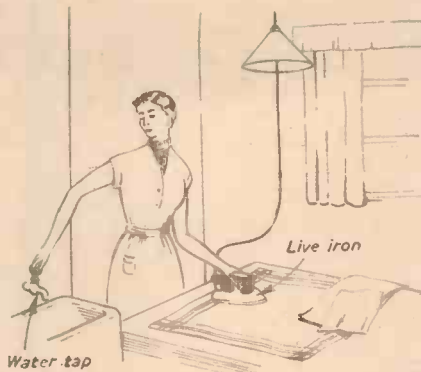
Fig. 5.—Showing how a housewife may obtain a shock from an unearthed iron.
