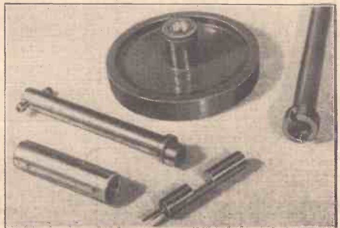
Fig. 5.—The flywheel, camshaft, ram and driving shaft.
