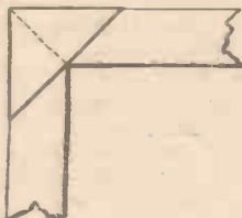
Fig. 2.—(Right) Strengthening the corner of the framework with a corner bracket.
