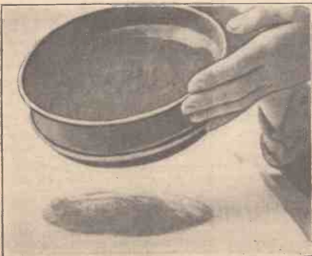
Showing the method of sieving a black pigment in order to obtain a fine powder of uniform particle size.
