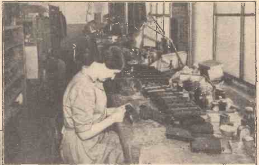
Fig. 1.—Manufacturing model locomotives : after painting, but before final assembly, the number and British Railways crest are applied, by means of transfers, to the model locomotive and tender respectively.
