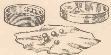
The balls may be picked up by means of a screwdriver having some Vaseline on the end. They should be laid on a piece of cloth and wiped clean so that they may be inspected for rust or pitting.
