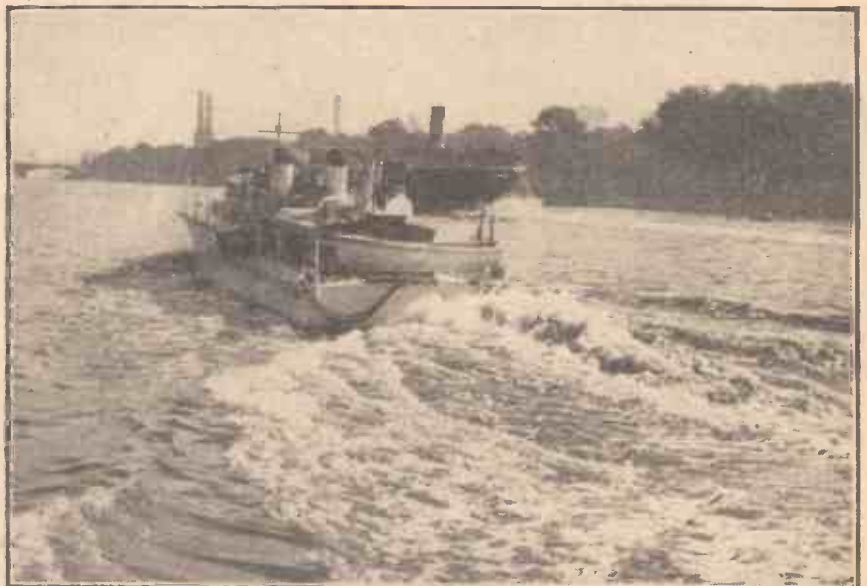
A demonstration motor launch fitted with Rover gas turbine engines was put through its paces on the River Thames recently and engineers were able to see the newly-developed engines (two of them in a 60ft. launch) in action. It is reported that the Admiralty has already placed an order for some of the engines, and it is hoped to develop them up to 200 h.p.
