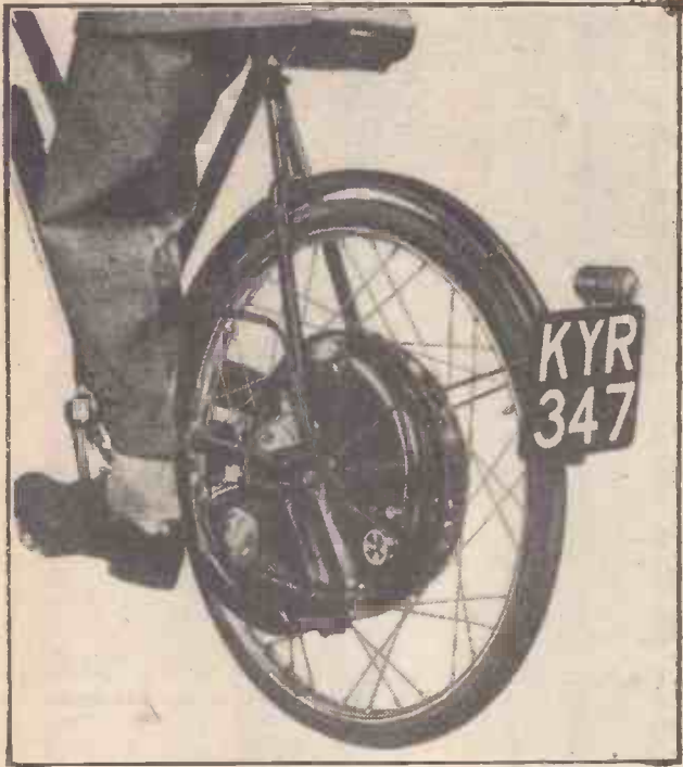
Fig. 6.—Showing the compact arrangement of the Cyclemaster. It is a complete back wheel which can be fitted to any machine.
