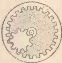
Fig. 97.—Internal toothed-gear wheel and pinion which maintains the direction of rotation.
