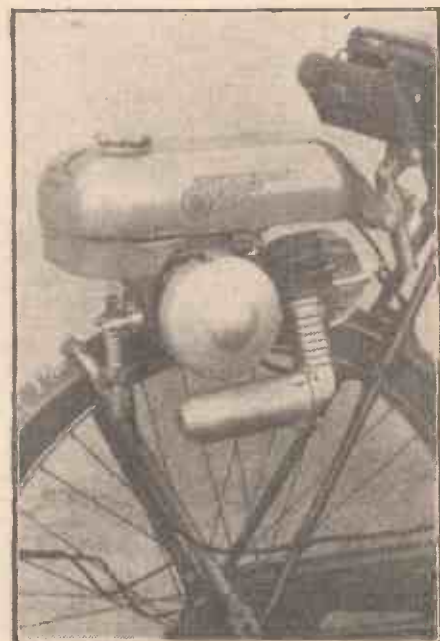
Fig. 5.—The Mini-Motor which is a friction drive on the back wheel. This engine can also be fitted to any cycle.
