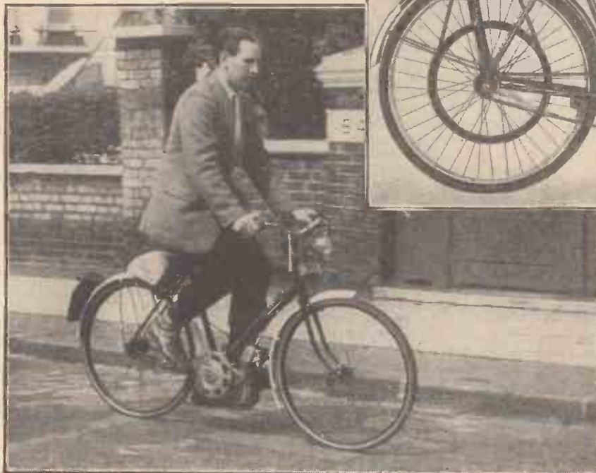
Fig. 9.—The Cucciolo "Micro-Motor" It is a four-stroke unit and is a chain drive on the rear wheel. It incorporates a two-speed pre-selector gearbox.
